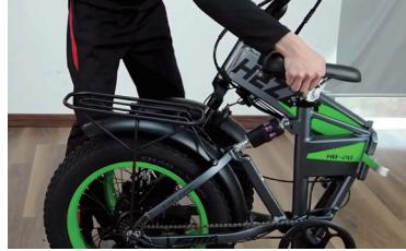
4. Release the clamp of the handbar
