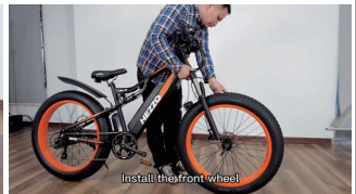
6. Install the front wheel
