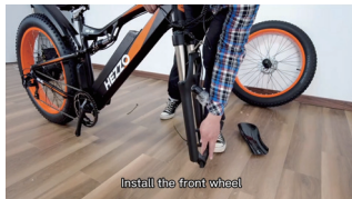
5. Install the front wheel
