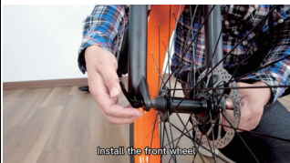
7. Install the front wheel
