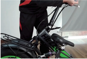
5. Fold the handbar and the pole
