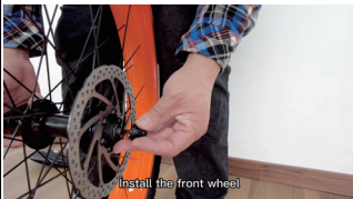
4. Install the front wheel
