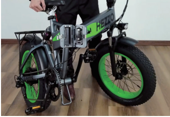
3. Unfold the bike (you may remove the battery from here too)
